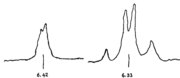
Figure 1. Temperature dependence of the nmr spectrum of trans -1-benzyl-2-phenyl-3- p -tolylaziridine (VIII).
